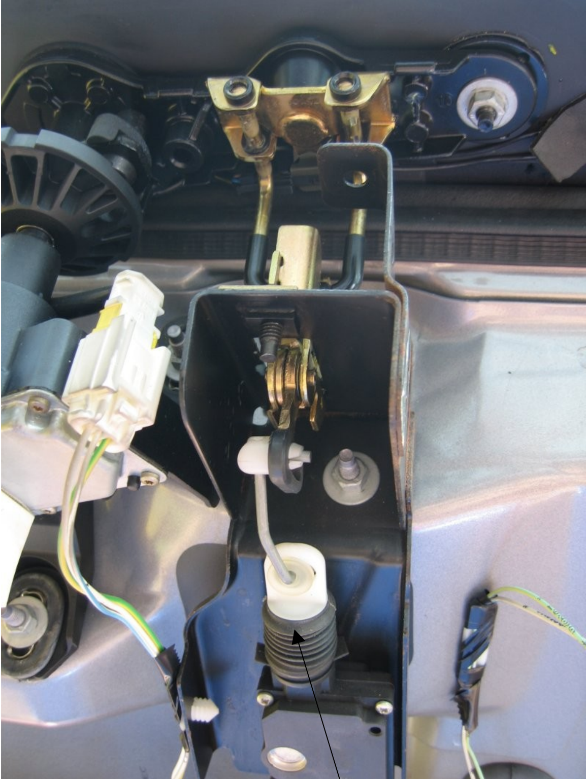
Picture of rear window catch and solenoid
