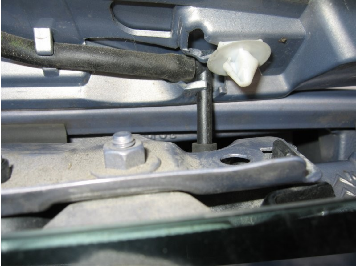
Photo of rear washer pipe.
